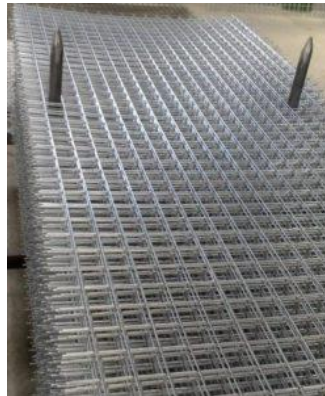
Figure 7.: Method of placing the products upon each other (Function: Prepare Packaging Unit)
