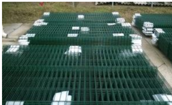
Figure 8.: Packing the product for transport (Function: Protect Product)
