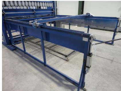
Figure 6.: Stacking (Function: Sustain Flow of Material)
